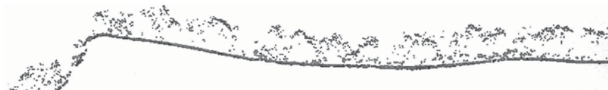
Fig. 13.4 A cross-sectional view of the canopy of a eucalypt forest in southeast Queensland, Australia, derived using laser scanning information from an aircraft flying at about 250 km/h at an altitude of about 1,200 m. The total distance across the image was about 500 m; the vertical and horizontal scales are the same. The solid line at the base of the image is the ground surface, which rises gently from right to left, then falls away quite sharply near the left hand end of the image. The dotted points represent the top of the vegetation canopy along the cross-section, measured in this case at about 1 m intervals; a contiguous set of 6–8 points in the upper reaches of the canopy might represent the crown of a single tree. The average height of the trees along this cross-section was measured on the ground as 24 m (from MBAC Consulting 2003, © Commonwealth of Australia, reproduced with permission)
